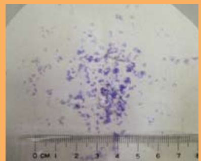
PM300 Easy Stripping for Higher Yield with 1~3mm of Stripping Flake Size
